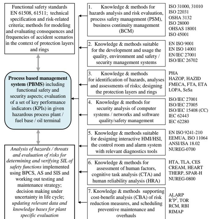
Figure 5. Process based functional safety and security management
