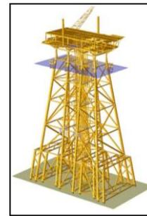
Figure 2. Offshore template (jacket) platform [10]
