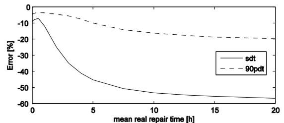
Figure 14. Standard deviation and 90<sup>th</sup> percentile of down time approximation error for hyperexponential real repair time
