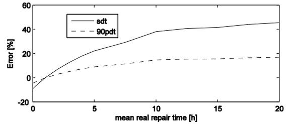
Figure 12. Standard deviation and 90<sup>th</sup> percentile of down time approximation error for Gaussian real repair time
