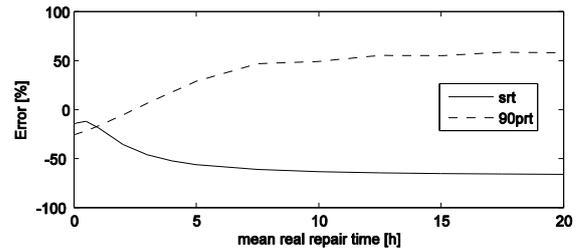
Figure 13. Standard deviation and 90<sup>th</sup> percentile of repair time approximation error for hyperexponential real repair time
