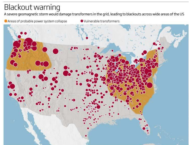
Figure 3. Map of expected blackout regions in USA after simulated CME with power from 1921 [8]
