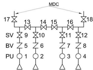
Figure 1. Technical scheme of the analyzed water pumping station: PU - pumping unit, BV - backflow valve, SV - stop valve on the discharge pipe (collector) (discharge gate), MDC - the main discharge collector, 1, 2, ..., 18 - numbers of pumping station elements
