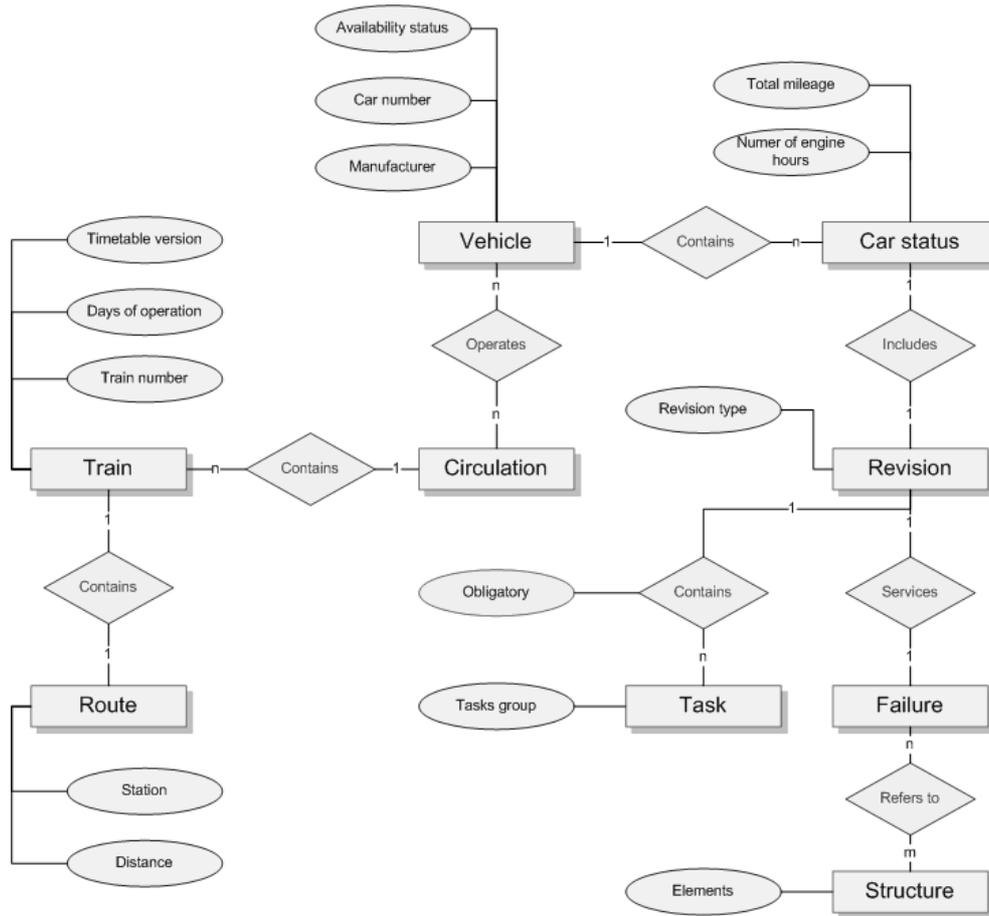
Figure 2. The model of railcar operation process shown as an entity-relationship-diagram [2]
