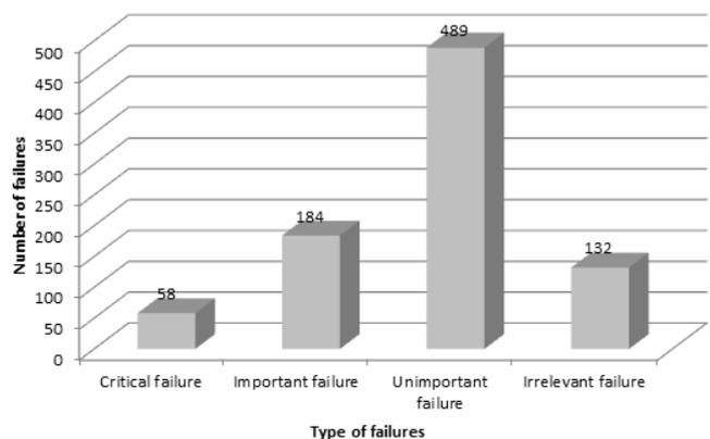
Figure 5. Distribution of failures types in terms of their influence on rail cars operational process performance [7]
