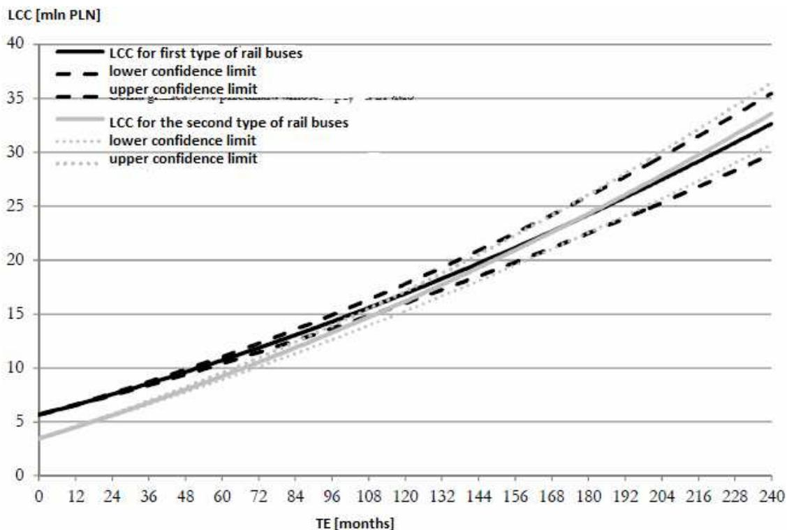
Figure 13. LCC for analysed types of rail buses [9]
