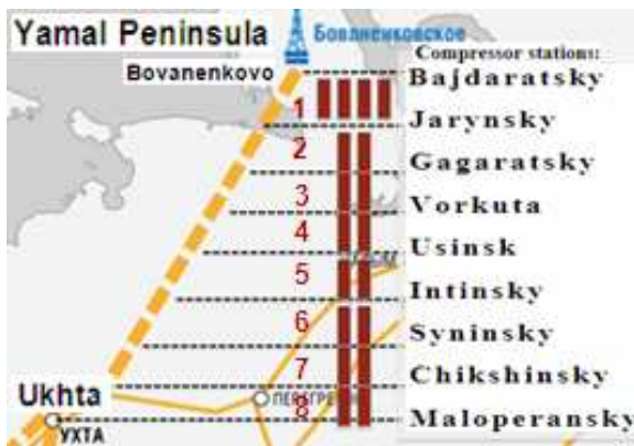
Figure 3. The analyzed fragment of the main gas pipeline
