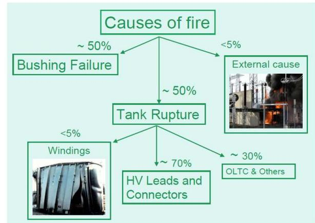
*Figure 4.* Causes of transformer fires
