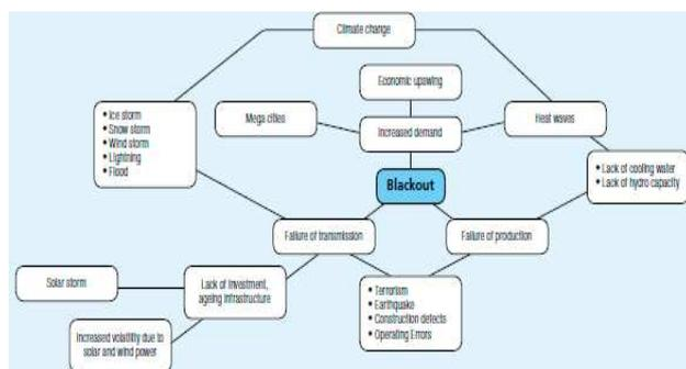
Figure 8. Potential causes of power blackouts according to [6]
