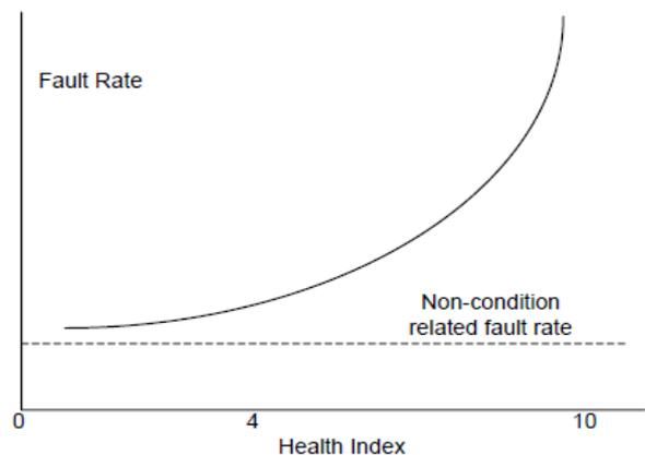
*Figure 5.* Health index related failure probability curve
