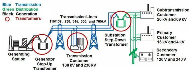
Figure 2. Typical electrical power network
