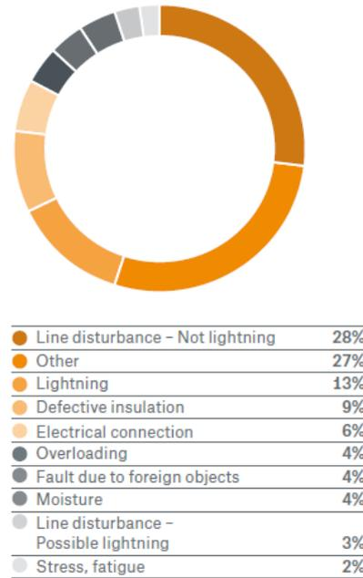
Figure 6. Causes of transformer failure according to [1]
