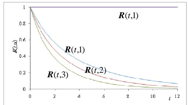
Figure 6. The graph of the container gantry crane reliability function  $\mathbf{R}(t, \cdot)$  coordinates
