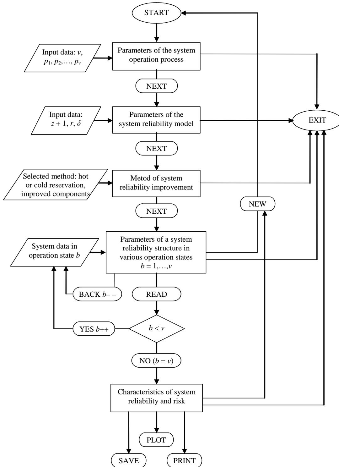
Figure 1. The scheme of the algorithm of the computer program for prediction of improved complex technical systems reliability and safety
